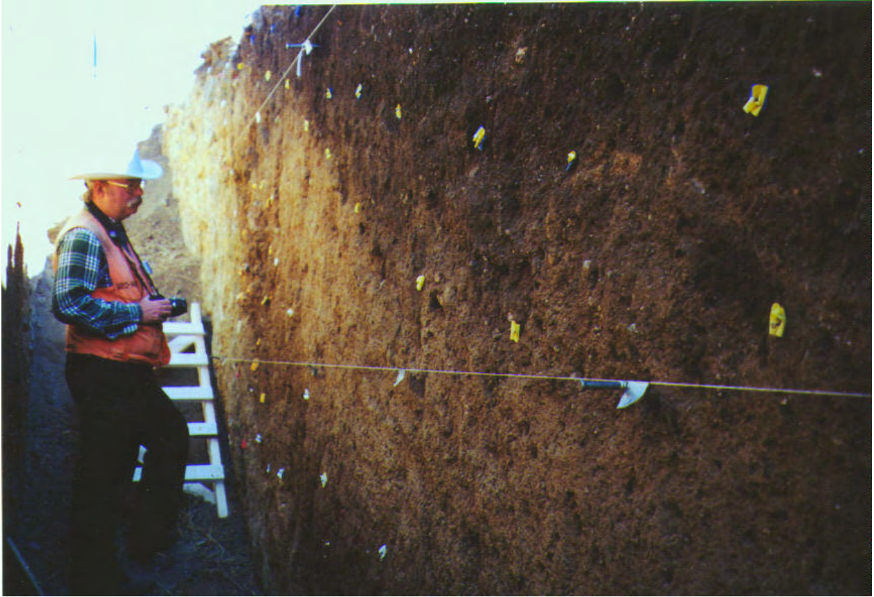
Fig. 18. Photograph of faults F1 and F2 in the Kagel Mountain trench (red flags in wall in front of J.P. McCalpin, near ladder). Fault F1 juxtaposes fairly intact, foliated granite (light tones at far end of trench) against light brown scarp-derived colluvium (left center) and dark brown soil A horizons developed on sandy slopewash (center and right). Note the upward drag of the colluvium (units 3 and 4) as they approach the fault.
