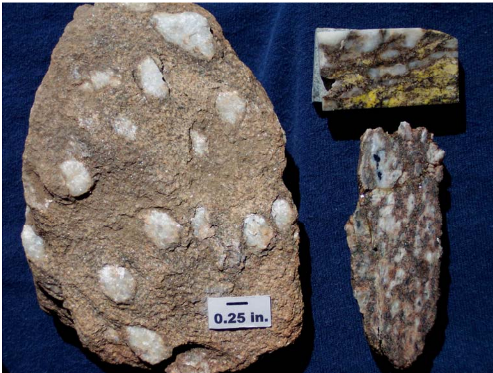
Figure 33. Hand sample, billet and slab of muscovite-sillimanite gneiss (Xmsg). Eyes are composed of sillimanite-quartz-muscovite. Billet is stained showing irregular distribution of alkali feldspar (upper right).
