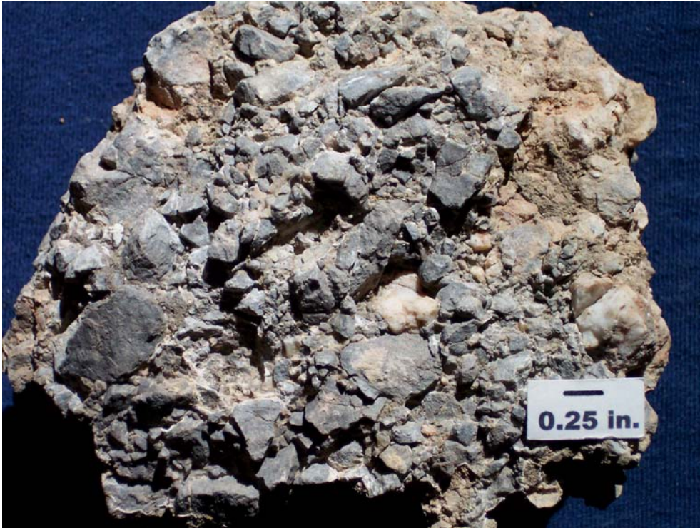
Figure 18. Close-up view of intensely shattered Paleozoic dolomite (gray) and minor chert (white) from the central Paleozoic landslide sheet (Td2ls) in the Dry Union Formation South Arkansas graben sequence (Td2).
