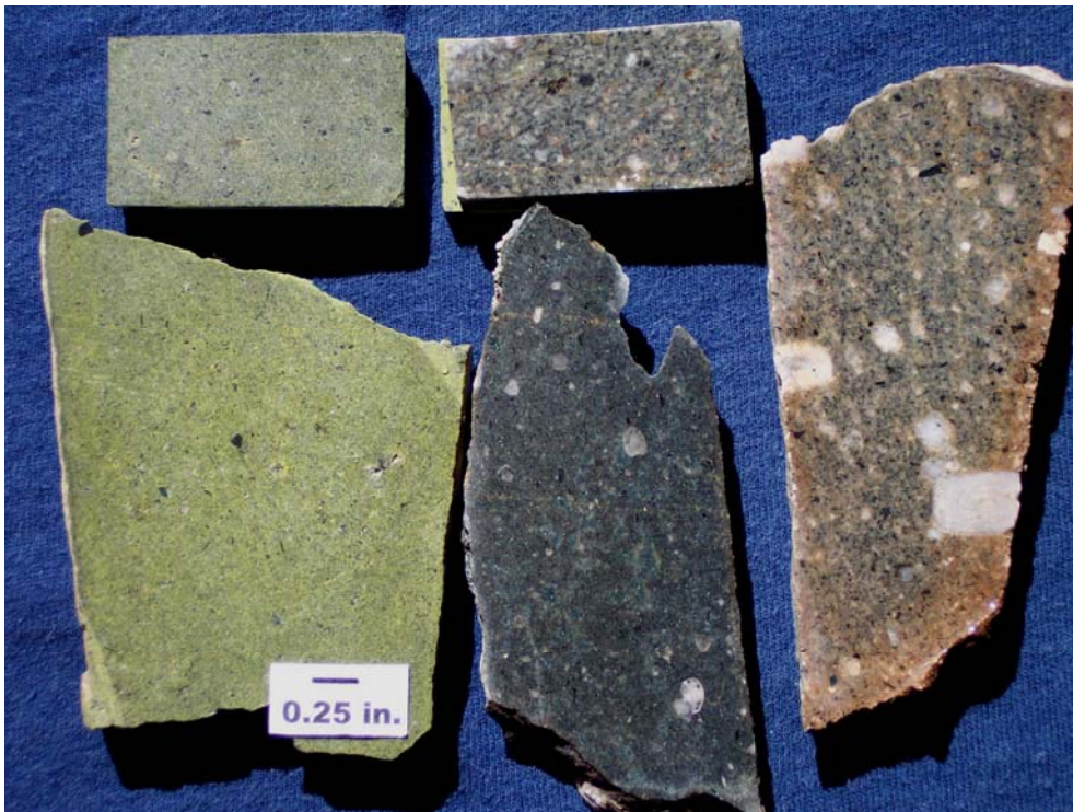
Figure 22. Billets and slabs of Tertiary quartz latite hybrid dikes (Tqlp) stained for alkali feldspar showing range of textures and xenocryst contents.
