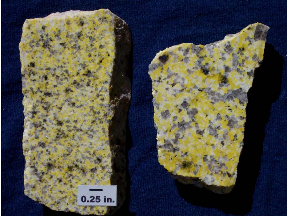
Figure 21. Slabs of North Fork border (Tnfb, left) and leucogranite (Tnfg, right) stained for alkali feldspar.
