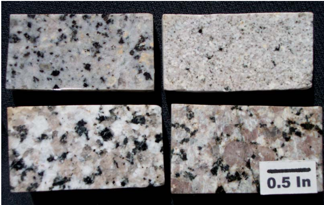
Figure 24. Billets of Mount Princeton pluton phases: Top, left and right- Tmpb border phases, porphyry and fine aplite; Bottom, left- Tmpm quartz monzonite subunit; Bottom, right- Tmpk porphyritic K-feldspar subunit.
