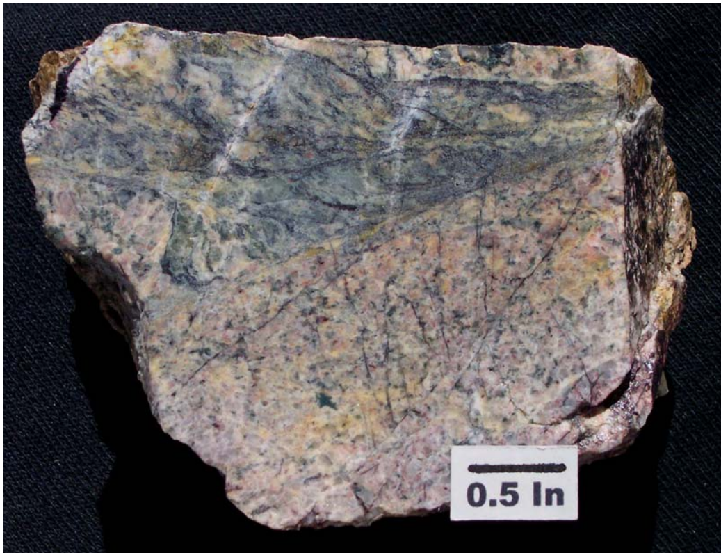
Figure 34. Proterozoic shear in YXg(?) with semi-ductile shear fabrics and superimposed quartz-hematite veining. From Hop Gulch area, northeast corner of the Buena Vista West quadrangle.
