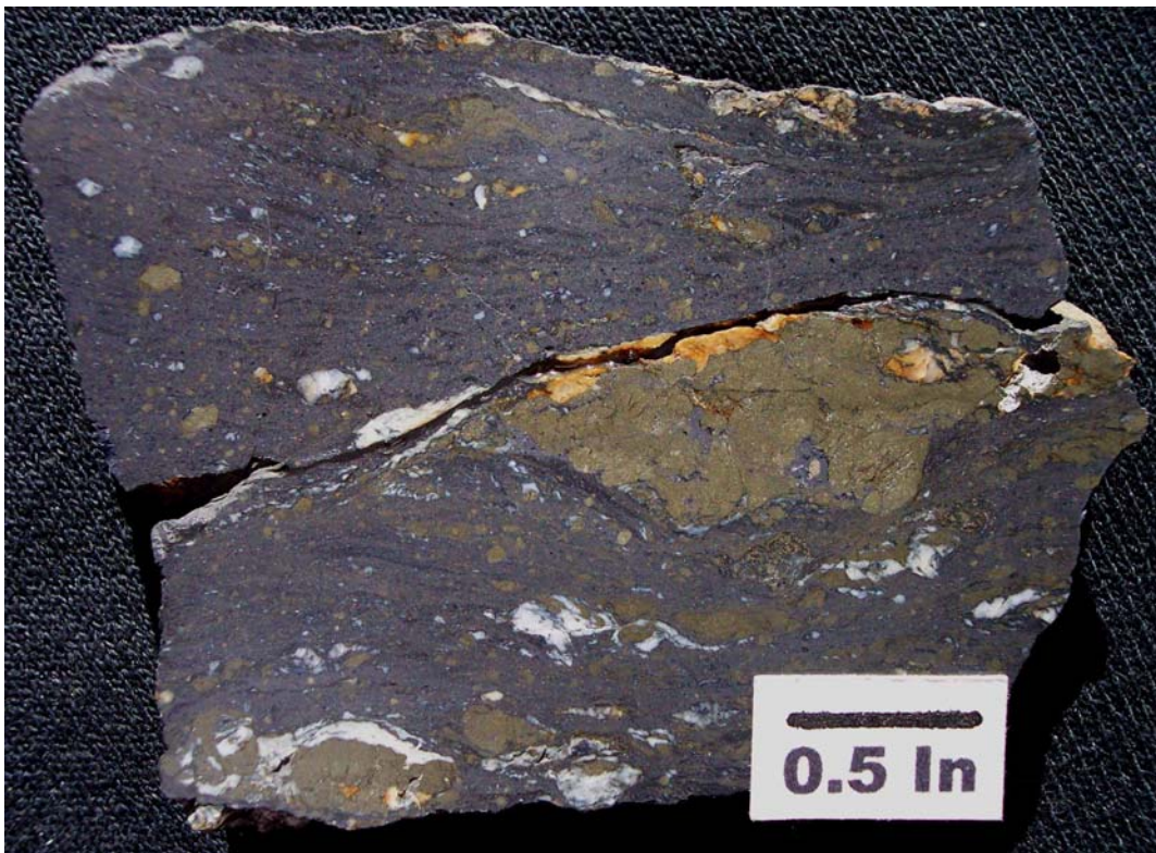
Figure 41. Slab of ductile sheared galena ore with mini-boudins of pyrite from the Latchaw Mine on Mount Princeton, Buena Vista West quadrangle. Sample 04B-120.
