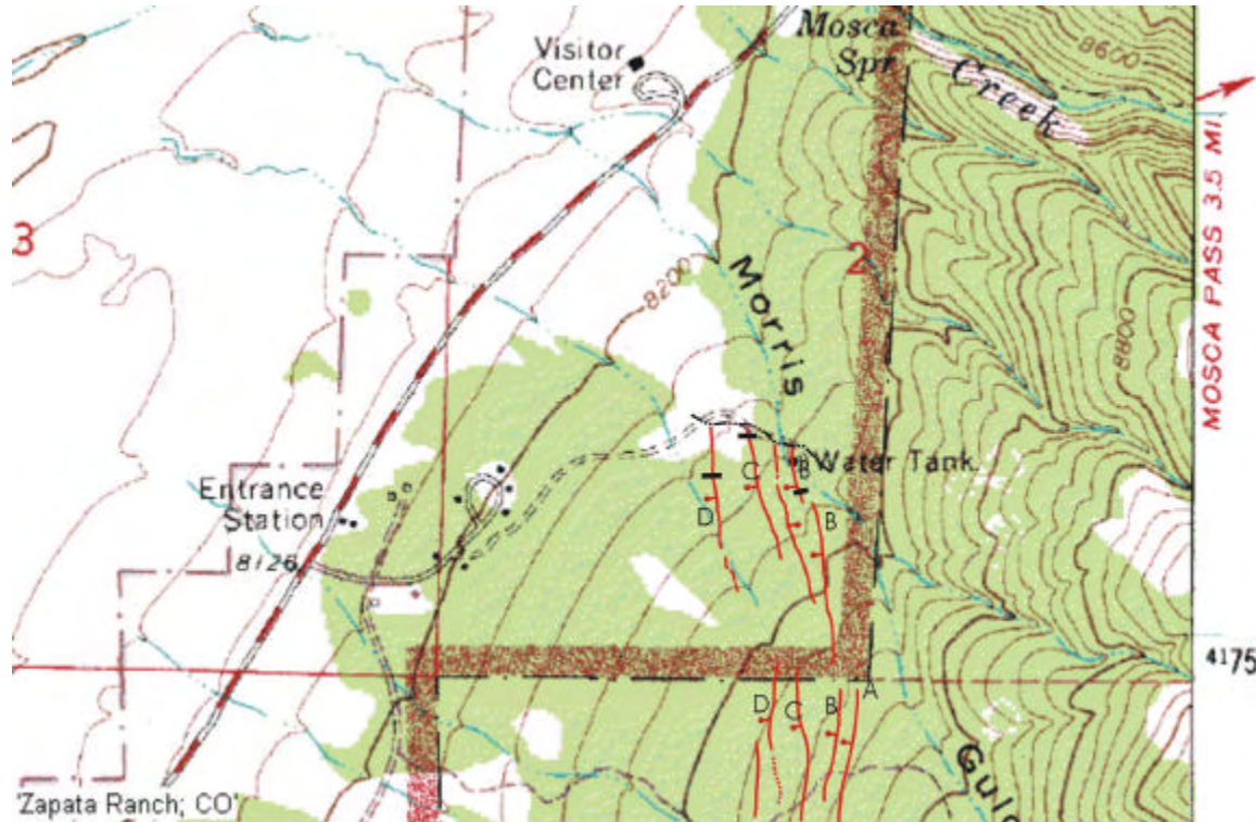
Fig. 5. Map of the fault scarps (A through D) mapped by students in the 2002 Field Methods course, at the mouth of Morris Gulch. The extension of scarp B north of the Water Tank is not shown. Black bars indicate 2002 trench locations. Base map from Mosca Pass 7.5' quadrangle, original scale 1:24,000.
